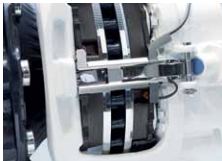
Disc Protector (optional): additional protection for trailer disc brakes in rugged applications.
