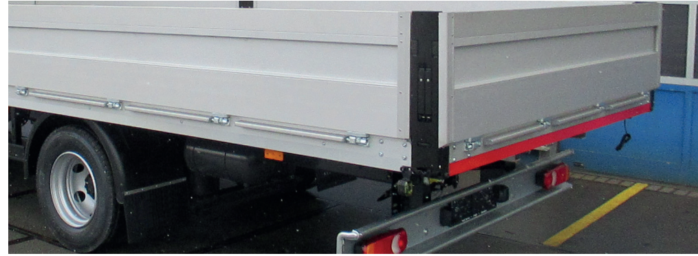
HESTAL SolidMaster 802 dropside pillars in 500mm (KTL coating)
