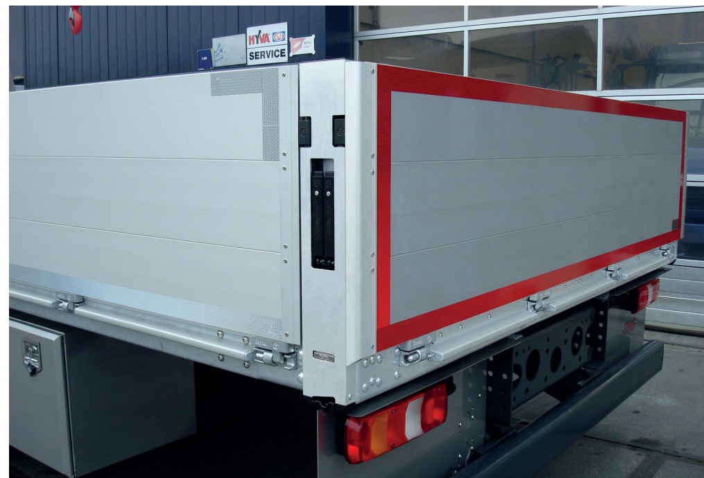
HESTAL SolidMaster 802 dropside pillars in 600mm (microZINQ®coating)
