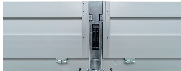
HESTAL SolidMaster 802M dropside pillar in 500mm
