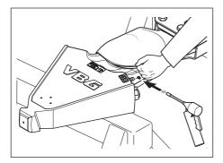
Lubricate the ball joint at least once a week with NLGI grease class 2 chassis grease (LB), Lithium + EP additive.
