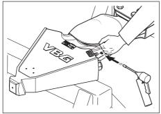
Lubricate with NLGI grease class 2 chassis grease (LB), Lithium + EP additive.
