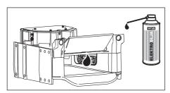
Lubricate the power plug with VBG Electro Oil.
