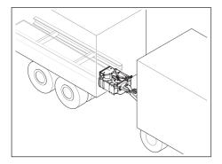
When checking for wear between the ball and ball seat, the coupling and drawbar wedge must be connected to each other.
