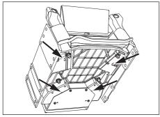
Keep the drainage hole on the underside of the coupling open.
