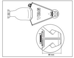
Clean the hole in the sensor. Never go deeper than 80 mm. Observe care to avoid damaging the sensor.
