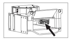
Blow clean the power points and hydraulics connectors inside the coupling by means of compressed air.
