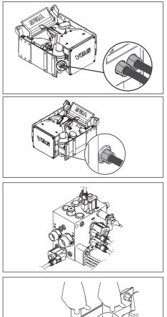
Check that air is not leaking from the air connections. Contact a workshop if there is any leakage.
